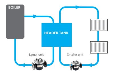
BoilerMagXT is typically installed on the return circuit as close to the boiler as possible. On larger systems, such as the one shown, smaller BoilerMagXT units may be installed elsewhere to give extra protection for radiators and pipework.
